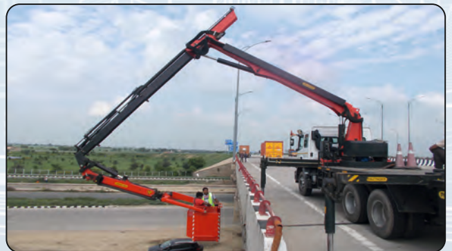
India: Bridge Inventory and Condition Survey Scope: Collection & Analysis of Bridge Inventory & Condition by Mobile Bridge Inspection Unit of 850 nos. of Bridges
